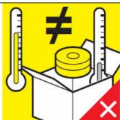
When packing, the goods and the environment must have the same temperature. Be careful to prevent premature condensation.
