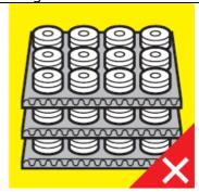
Avoid direct contact between metal and wood, cardboard or paper! Use intermediate layers made from VCI carrier materials.
