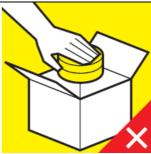
Items to be packed must not come into contact with sweaty hands. Always use clean gloves for unpacking/packing of the parts that must be stored.
