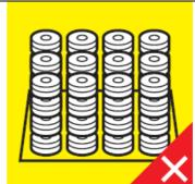
If parts are purchased in high quantities, they are provided (if required) with VCI interlayers. When repacking the parts, VCI interlayers must be applied again.
