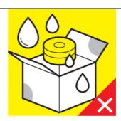
Always unpack/pack the parts in a cleaned area, free of excessive moisture. In case of storage of the parts for more than 12 months, the packaging should be inspected, and parts protections means applied ex-novo.
