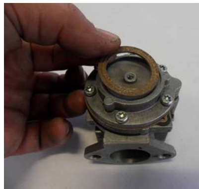
Figure 6 Cork sealing mounting
